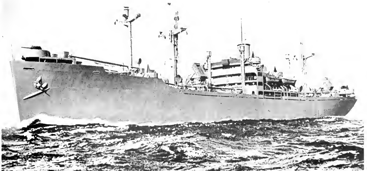
VICTORY SHIP, CLASS VC2-S-AP 2, FITTED FOR WAR SERVICE. Rigged model USNM 313023 shows the basic design of the class. (U.S. Maritime Administration photo 3969.)
